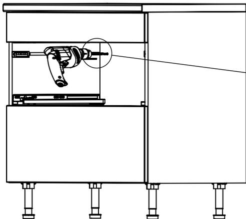
Loch bohren - Ø8mm
